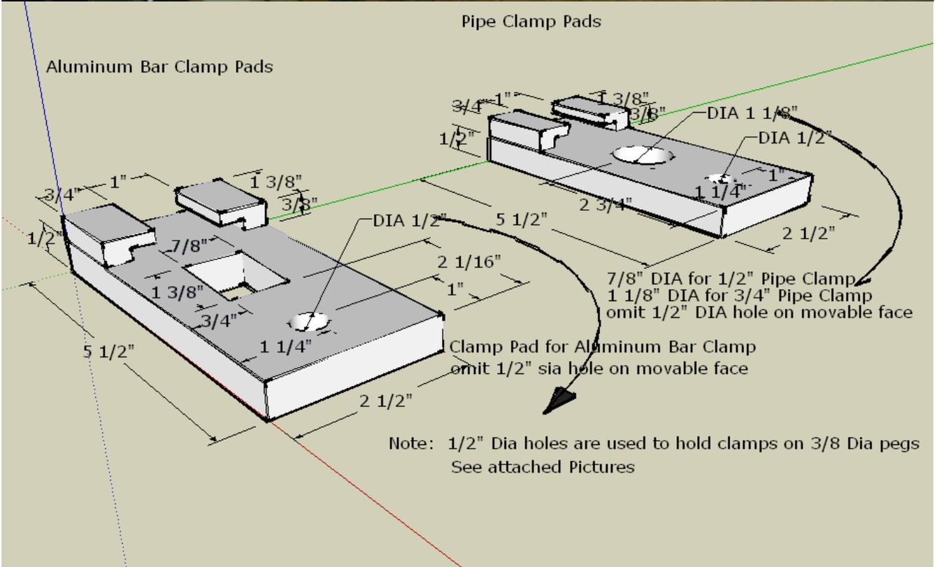
The basic pad is the same for pipe and bar clamps.
